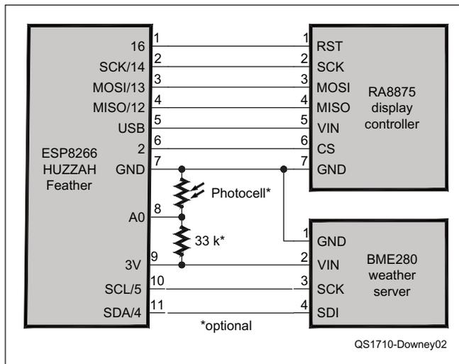
**Figure 2** — Wiring diagram of the main HamClock components.
