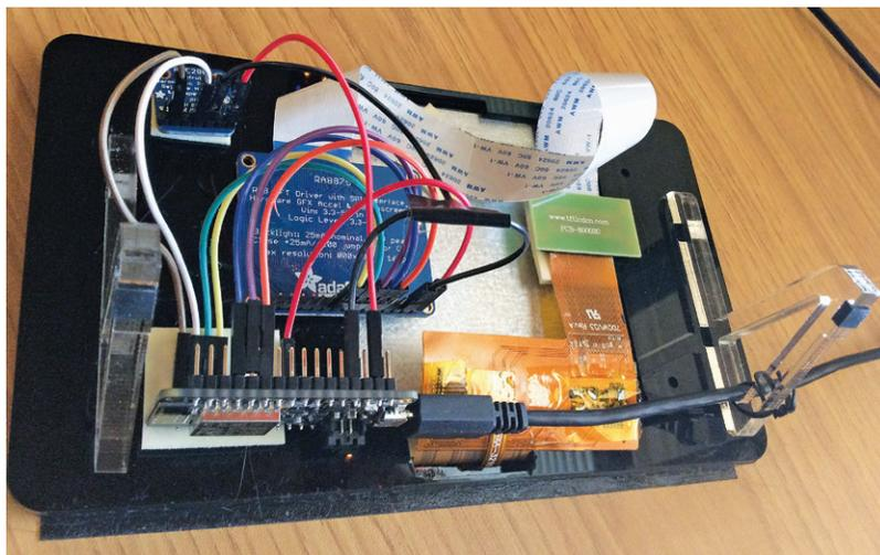
**Figure 3** — The rear of the HamClock shows how the main components are adhered to the back of the bezel and shows the wiring using female-female jumper wires.
